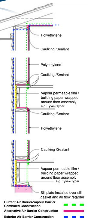
Alternatively to sealing every joint in the air barrier system as required by prescriptive requirements you can blower door test your building to CAN/ULC-S742 or ASTM E2357. IF the blower door test meets the air changes per hour requirement this will also meet the Building Code requirements.
